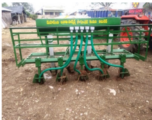
A new machine for the plantation of Turmeric saplings
